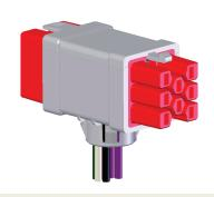
Low-profile device provides quick connection to light fixtures. Snap-in ½" trade knockout design can be field or factory installed. Integrally moulded for superior strength and reliability.
